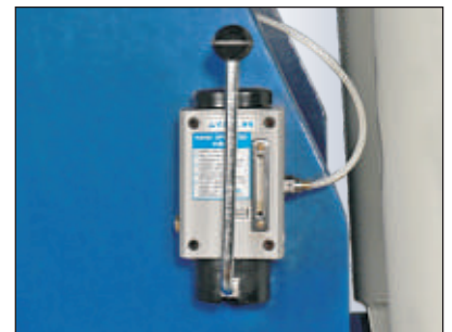
Manual lubrication system
