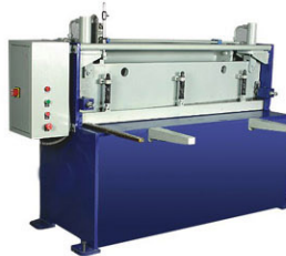
Fix Rake Angle Hydraulic Shear Range : 2 MM. x 1500 MM to 10 MM. x 1500 MM
